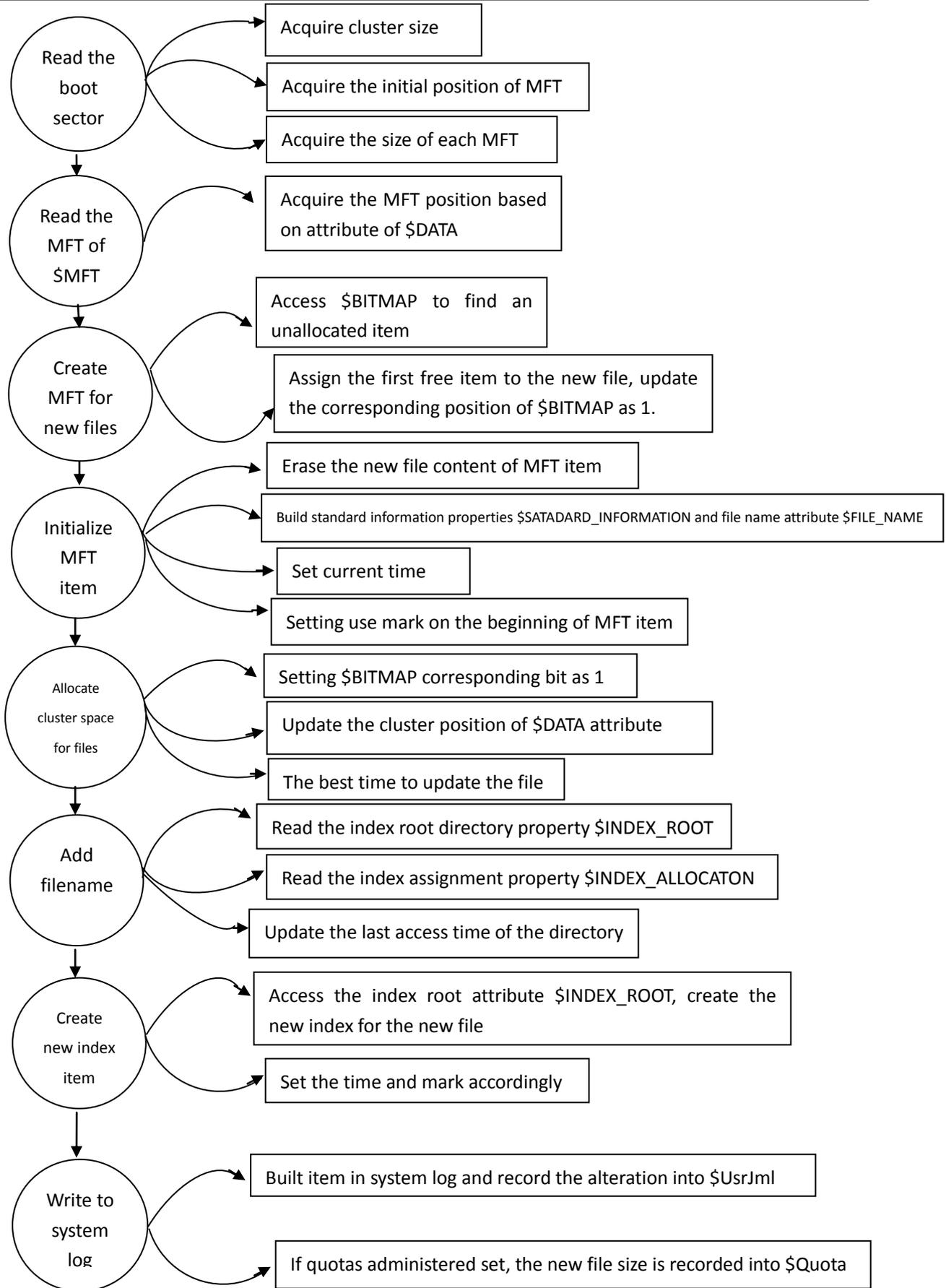
From the above flow, we can see the process of writing data is also the process of updating mapping table. The abnormal power-off during this period still can affect the complete updating of mapping table.
